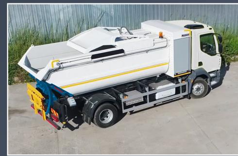
Thanks to its small footprint yet impressive 9 m<sup>3</sup> capacity, the CITYPACK is the perfect waste compactor for inner city & urban areas. The CITYPACK is equipped with a fully hydraulic bin lift system, capable of handling bins from 120 litre to 240 litre capacity, thereby increasing the flexibility & speed of loading.
