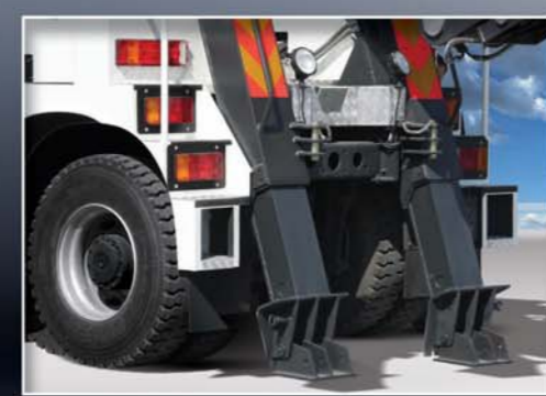
DENGE AYAKLARI SUPPORTING LEGS TO PROVIDE MAXIMUM STABILITY
